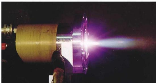
Fig 1: Steam plasma torch in operation
